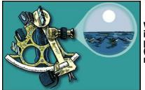
What makes a sextant so useful in navigation is its accuracy. It can measure an angle with precision to the nearest ten seconds. (A degree is divided into 60 minutes; a minute is divided into 60 seconds.)
